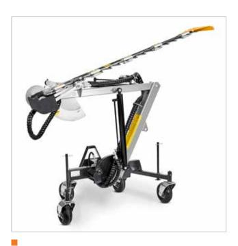
**Cut the hedge from the driver's seat of the Park Ranger 2150** The hedge cutter is hydraulically controlled and has a large range, a vertical cutting height from 0-320 cm and a horizontal cutting height of up to 210 cm.
